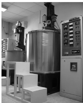
Fig. 4 Large homemade furnace with three-zone resistive heating for the crystal growth of LBO
