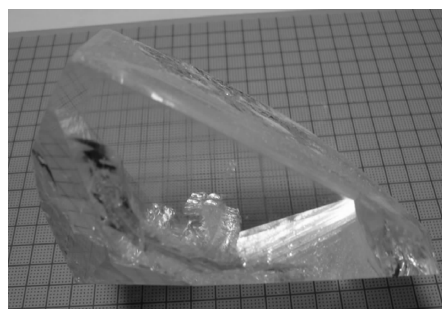
Fig. 6 LBO crystal with the size of 170 \text{ mm} \times 160 \text{ mm} \times 79 \text{ mm} and the weight up to 1 596 g
