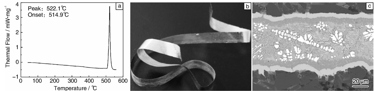
图 14 SiCp/Al 复合材料用 Al 基中温钎料的 DSC 曲线(a)，钎料薄带的照片(b)，钎焊组织的 SEM 照片(c) Fig. 14 DSC curve of Al-based medium-temperature soldering used for SiCp/Al composite(a)，Photo of Al-based soldering thin tape(b)，and SEM micrograph of SiCp/Al composite soldered with Al-based medium-temperature soldering(c)
