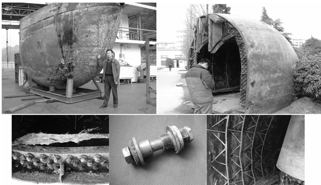
图6 俄罗斯“956 型现代级”导弹驱逐舰钛合金球鼻艏 Fig. 6 Titanium bulbous bow of Russia “956-type modern class” guided missile destroyer
