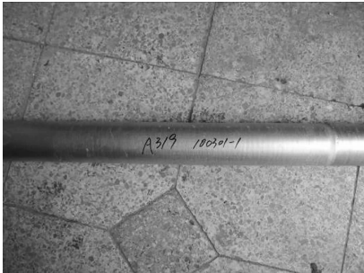
图 9 环缝式电磁搅拌制备的 A319 铝合金坯料 Fig. 9 A319 alloy billet prepared by annulus electromagnetic stirring
