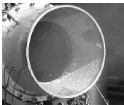
图 2 C/C-SiC 燃烧室和喷管及热试车 Fig. 2 C/C-SiC combustion chamber, nozzle and hot-firing tests
