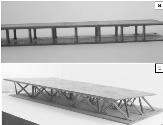
Fig. 8 Carbon fiber-reinforced sandwiches with (a) columnar and (b) pyramidal lattice truss cores
