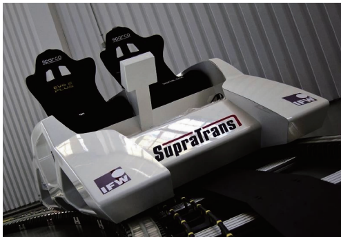
图 5 德国“SupraTrans II”高温超导磁悬浮车 [22] Fig. 5 HTS Maglev test vehicle in Germany, “SupraTrans II” [22]
