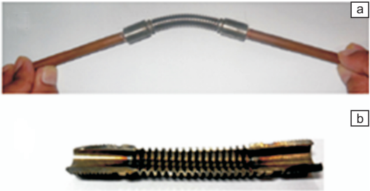
图 4 金属波纹管柔性热管照片(a)，波纹管截面照片(b) [12] Fig. 4 Photographs of the flexible heat pipe connected with bellows (a) and cross-section of the bellows section(b) [12]
