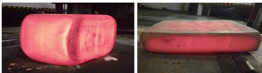
Plate size: 390 mm×1970 mm×3100 mm Result of ultrasonic testing: \Phi 1.2
