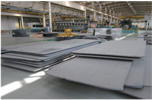
图 11 西部钛业公司制备的低成本高强度钛合金板材 Fig. 11 Low-cost high strength Ti-alloy plates produced by Western Titanium Technology Co., Ltd.
